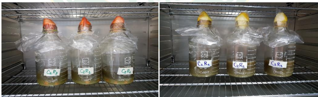
Figure 9 Stalk juice fermentation: immobilized yeast (left) and free cell yeast (right).
