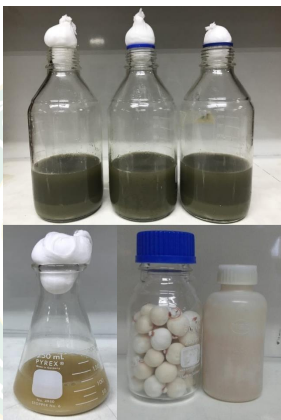
Figure 8 Readily fermentable sugar from corn stalk juice (top) free cell yeast used for fermentation (lower left) and immobilized yeast (lower right).
