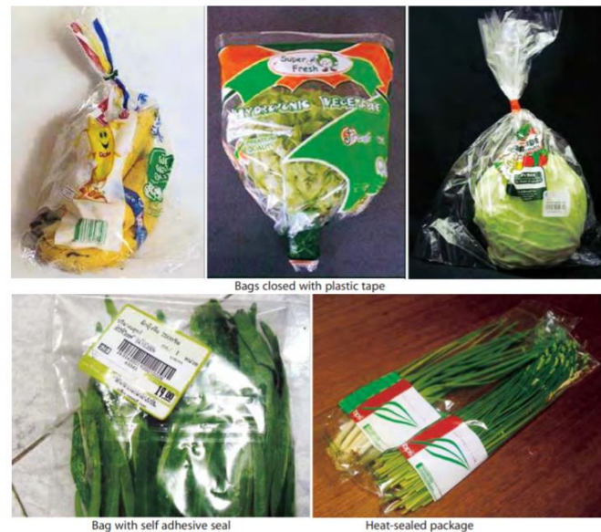
Figure 8 Produce packed in PE and PP bags that are sealed using different methods.
