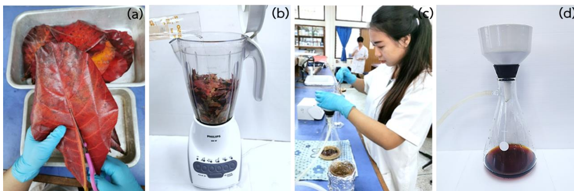
Figure 16 The extraction processes (a) Cut to small pieces, (b) The sample mixed with methanol by using a blender, (c) The vacuum filter was separated solid and liquid and (d) The pigments extraction
