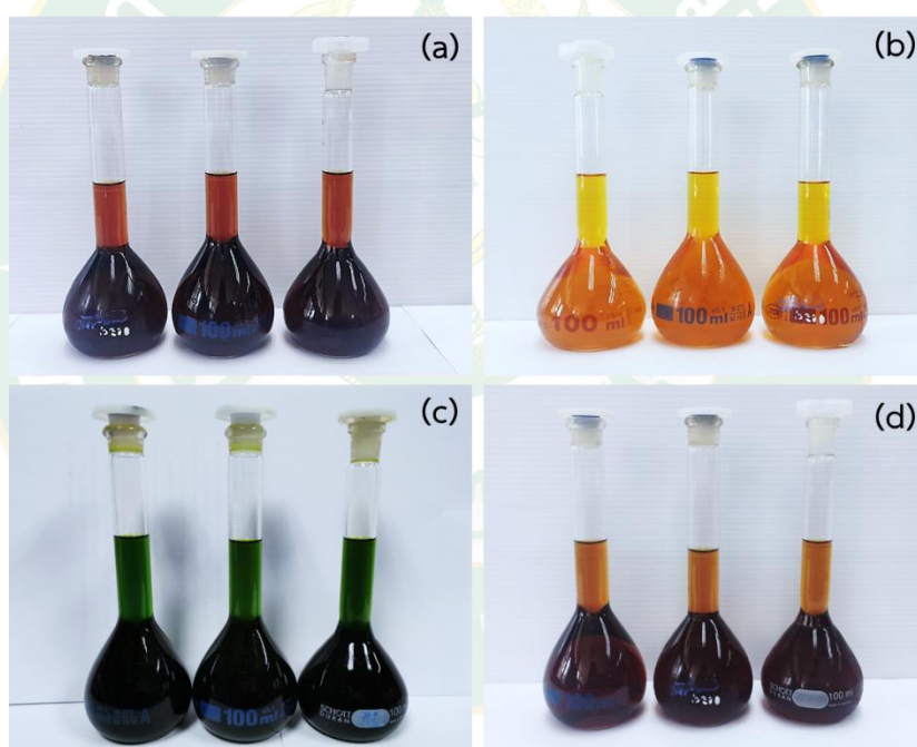
Figure 17 The natural dyes from (a) Indian almond, (b) Yellow cotton, (c) Longan and (d) Inthanin bok
