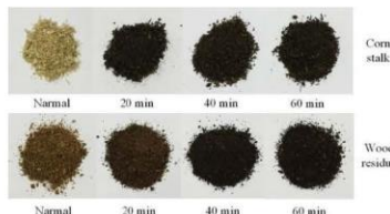
Fig.7 Color of corn stalk and wood residue at different torrefaction time.
