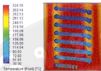
Figure 6. Temperature distribution in the re-burning kiln with water flow rate at 10 LPM.
