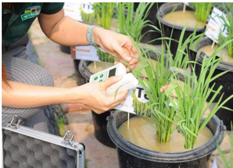
Figure 5 Measuring SPAD value on YEB of the rice plant
