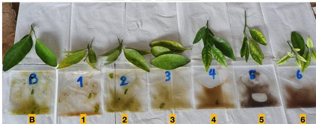
Figure 21 The color of the testing solution of CGD (1-6) compared to baseline or no symptom (B)
