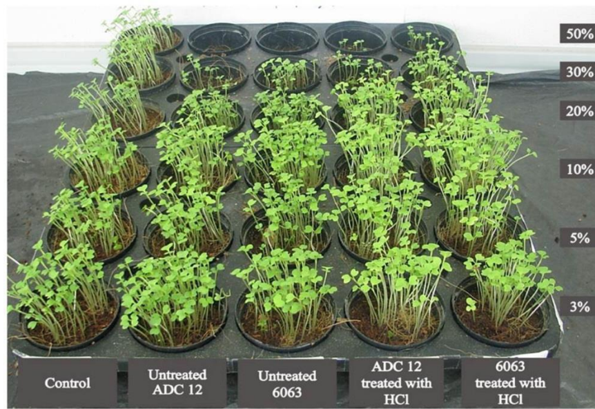
Figure 35 Untreated and treated dross of Chinese cabbage with HCl in 13 days
