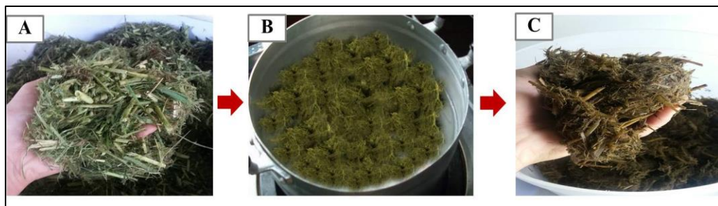
Figure 23 Thermal pre-treatment of para grass
