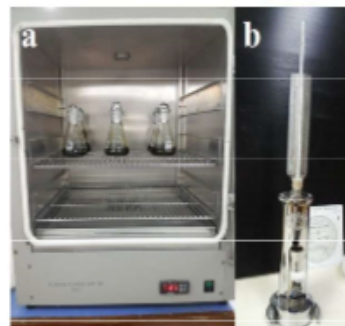
Fig. 3. Batch bioethanol experiment (a), Ebulliometer (b).
