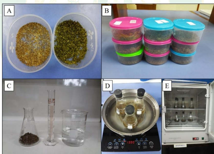
Figure 17 Biological pretreatment; Feeding termite with materials (A and B); Adding 100 mL of distilled water and boiling for 1h (C and D); Enzymatic hydrolysis (E)
