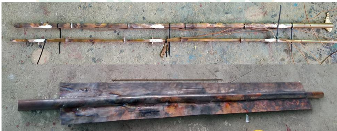
Figure 30 The riser tube phase change material with thermocouple.
