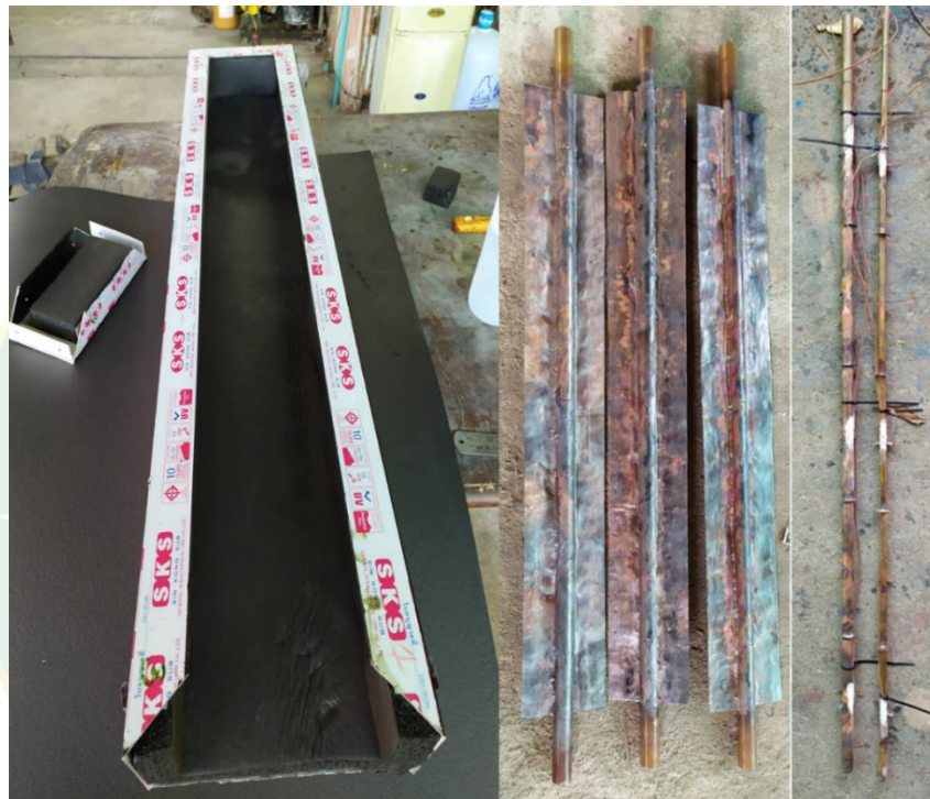
Figure 21 The novel solar collector frame, copper plate and riser PCM.
