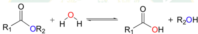
Figure 2. 8 Chemical reaction of hydrolysis
