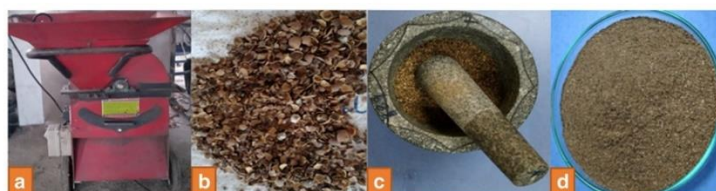
Fig. 2 a Shredder machine. b The samples after using the shredder machine. c Mortar and pestle. d The smaller size samples
