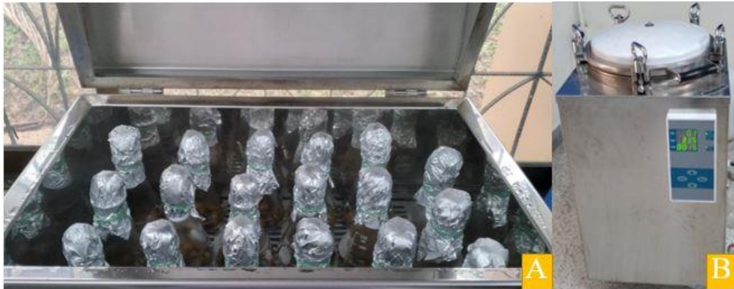
Figure 3. 5 Pretreatment process; boiled sample (A); Autoclaved sample (B)
