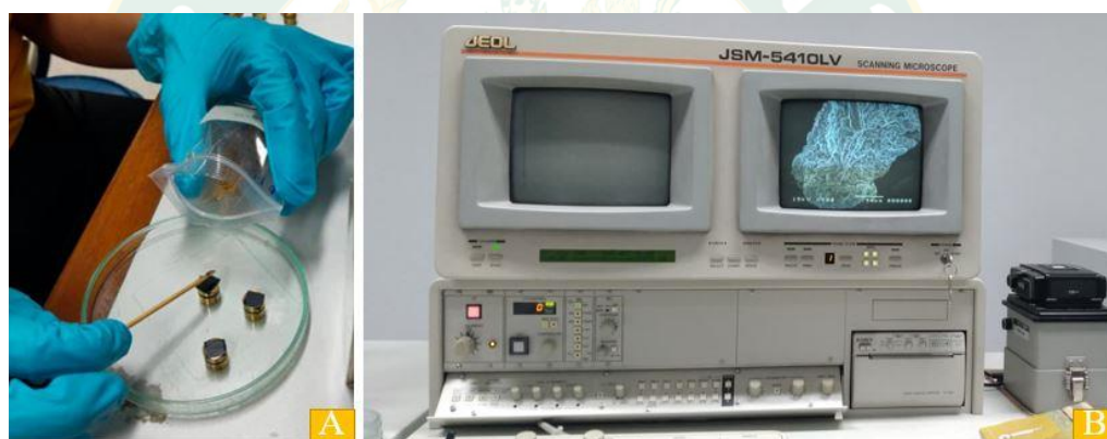
Figure 3. 8 Sprinkle of sample in pure gold (A); Scanning electron microscope equipment (B)
