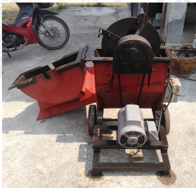
Figure 13 Making powder by blender about 1-2 mm of samples
