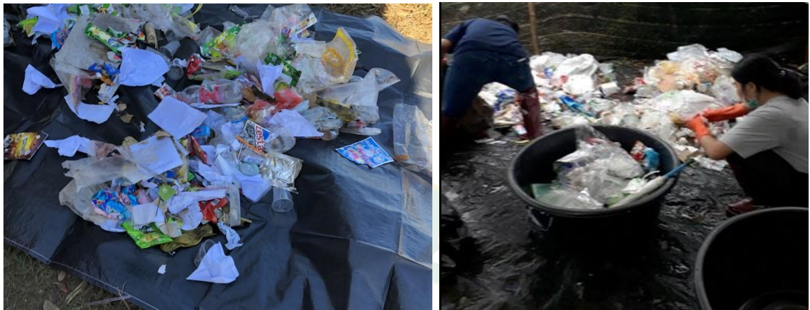
Figures 1 The sampling process (Quartering method)
