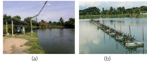
Figure 1 Aquaculture pond (a) Air Stone aeration system (b) Turbine aeration system
