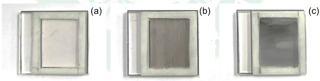
Figure 29 Counter electrodes: FTO glass (a), FTO glass with graphite (b), FTO glass coated with platinum (c)
