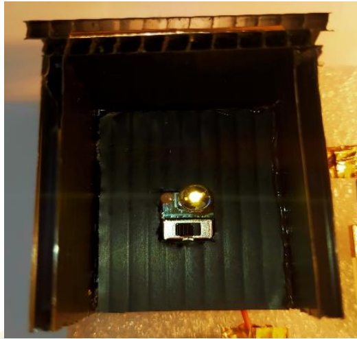
Figure 62 LED light powered by DSSC
