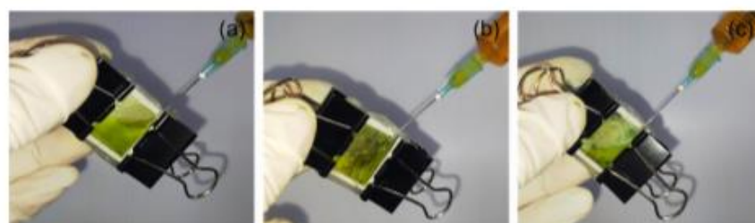
Fig. 7 Injection of electrolyte to different counter electrodes: FTO glass (a), FTO glass with graphite (b), FTO glass coated with platinum (c)
