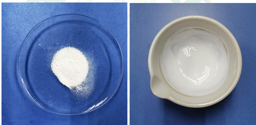
Figure 27 Preparation of TiO 2 paste: TiO 2 nanoparticles powder (left) and mixture of TiO 2 powder and 5% acetic acid (right)
