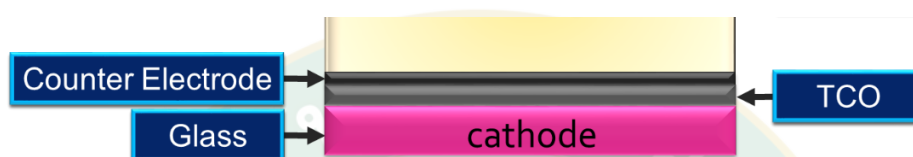
Figure 3 Composition of counter electrode
