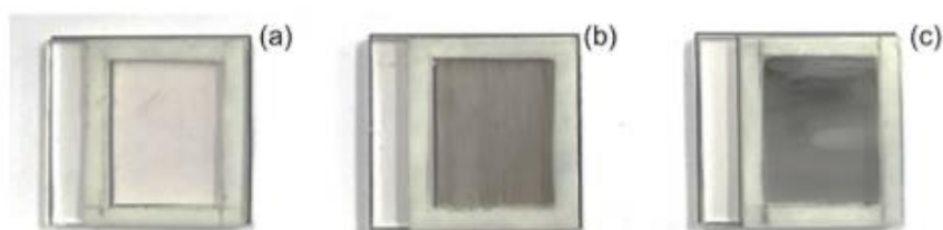
Fig. 5 Counter electrodes: FTO glass (a), FTO glass with graphite (b), FTO glass coated with platinum (c)
