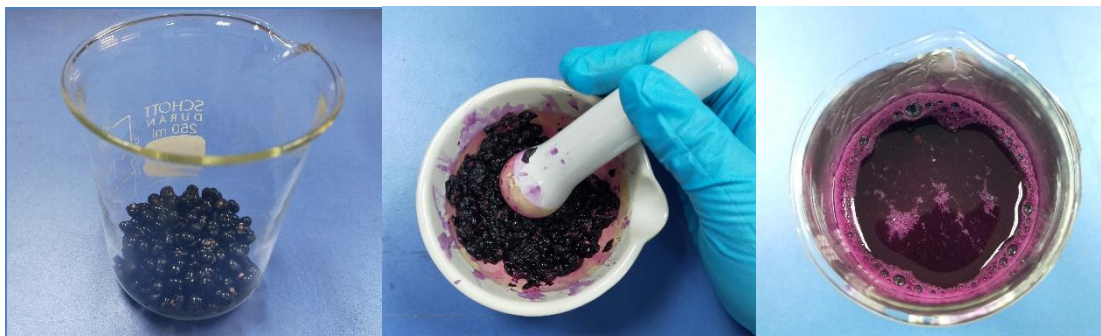
Figure 18 Raw materials are washed, dried at room temperature then weighed (left), then crushed with mortar and pestle (middle), mix with solvent (right)
