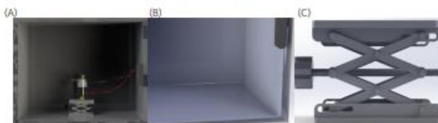
Figure 3 (A) Door and cold plasma cabinet (B) Round corner and (C) Sample stage
